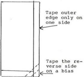
This allows expansion and contraction with the least damage
